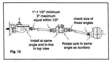
If there is more than one driveshaft between the device and the rear axle, install the driveshafts as outlined earlier with a 1 to 1 1/2 degree u-joint operating angle on the input end of each shaft. Then rotate the axle so it is on the same angle as the last fixed shaft. The u-joint operating angle on each end of the last shaft will automatically be equal. (See Fig. 14)
