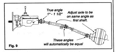
If there is an offset in the installation of the axle, make sure it does not create too large of a compound u-joint operating angle. Whenever possible, mount the axle directly in line with the first coupling shaft (when viewed from the top).
