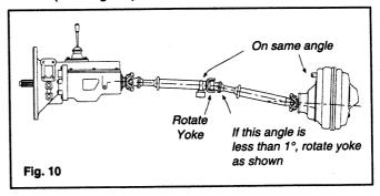
On applications having more than two shafts, mount the first coupling shaft as outlined in the preceding example, and each additional coupling shaft at a 1 to 1 1/2 degree u-joint operating angle to the previous coupling shaft.
