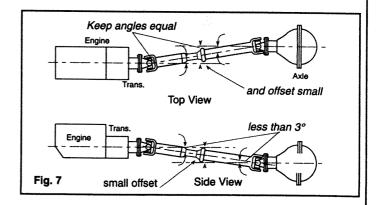
NOTE: Centerlines of transmission and axle must be parallel in both top and side views to use this method of determining true U-joint operating angle. Please contact the Drivetrain Service Division Spicer Universal Joint product manager at 419-866-3900 if you have an application where the components cannot be installed with their centerlines parallel.
