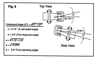
Do the same for the other end of the shaft. Compare the resultant calculated u-joint operating angle for each end. They should be EQUAL within one degree. If they're not, the driveshaft will vibrate.
