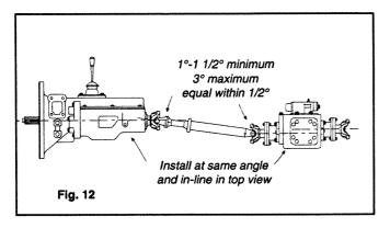
If there is only one driveshaft between the device and the rear axle, rotate the rear axle (using shims in the appropriate place) so it is the same angle as the device. This makes the u-joint operating angle at each end of the driveshaft equal. (See Fig. 13). Check the size of the u-joint operating angles to determine if they meet recommendations.
